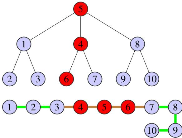
Fig. 1. GTQ protocol which uses a logical tree topology (top) mapped onto a bus-like network (bottom). The blue circles represent (nodes hosting) replicas. The (nodes hosting) replicas in red have failed.
